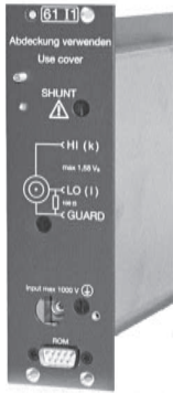
Current channel 6111 with triaxial socket for shunt identification
